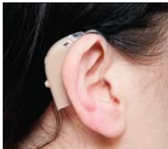
**Receiver-in-the-ear (RITE) or loudspeaker-in-the-ear BTEs** (not currently available on the NHS) have a clear tube with a wire inside, which runs from the BTE to a
