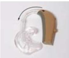
This picture (left) shows the earmould put back the wrong way round. Make sure the curve of the earmould goes the same way as the curve of your hearing aid (right).
